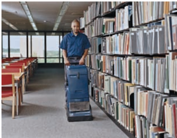
Power Vacuuming and Pile Lifting
